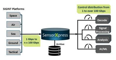
Unlike today's top-end wideband recorders, SensorXpress can stream data simultaneously on disk and off disk at over 100 Gbps, allowing for a consumption of a larger volume of SIGINT data from multiple sensors. SensorXpress also stores data at a much higher density without quality loss – close to Petabyte in just a 2U form factor. Being sensor, analysis tool, and spectrum agnostic allows you to extend the useful life of your existing SIGINT/ELINT infrastructure while maximizing its capabilities.
